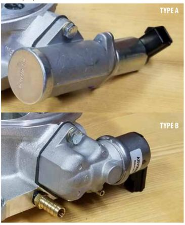
2. Remove the existing IAC Valve/Motor from throttle body. Remove any remaining gasket material and clean IAC flange on Throttle Body. If equipped, use the provided plug to block off passenger side vacuum port. (See red arrow)
