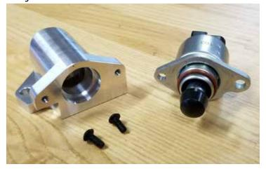
4. Align the new IAC adapter and gasket to the IAC flange on the throttle body. Install IAC adapter with provide 1/4"-20 x 5/8" hex bolts and washers. Do not over-tighten.
