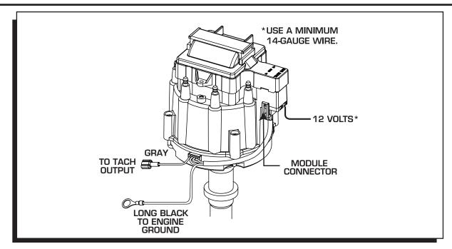
Figure 5 Connecting the Module and Tach Lead.
