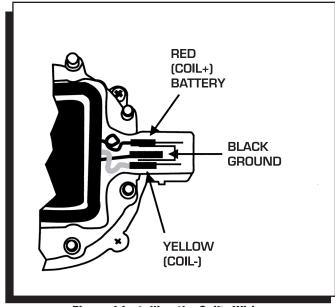
Figure 4 Installing the Coil's Wiring.
