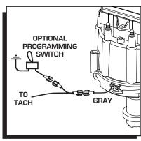
Figure 7 Setting the Rev Limiter
