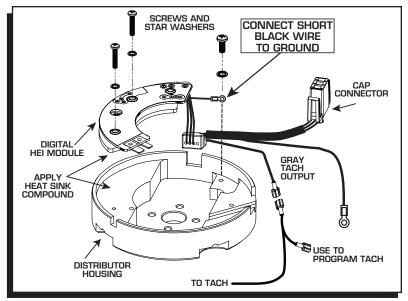
Figure 1 Installing the Module.
