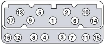
Figure 3 - Cylinder Head Bolt Torque Sequence Torque Bolts to 65 ft./lbs. in Three Steps (40-55-65)
