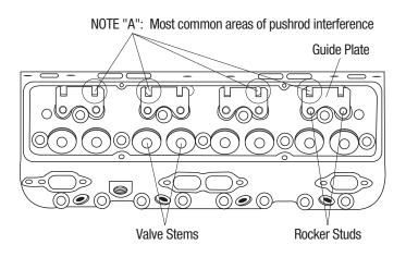
Figure 4 - Pushrod Guide Plate Clearance
