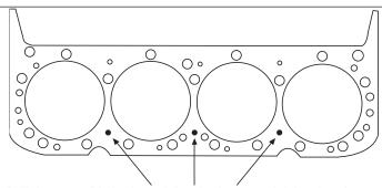
Drill three .125" holes in each head using 400 c.i.d. head gasket as a guide. **DRILL ONLY THE THREE LOWER STEAM HOLES** (closest to the spark plugs) as indicated. Drill straight into the head (90° from the deck) until the drill breaks through into the water jacket (about 9/16").
