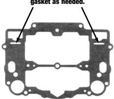
**NOTE:** Some carburetor tops have cast-in baffles near the slots in the gasket, as shown in the figure to the left. If this is the case with your carburetor, the gasket may need to be trimmed to properly fit over the baffles. Trim the gasket as shown.
