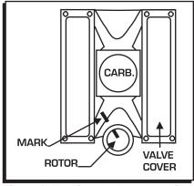
Figure 1 Marking the Rotor Location.
