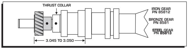
Figure 13 Replacing the Distributor Gear.
