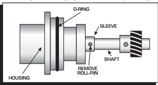
Figure 7 Removing the Retaining Sleeve.
