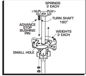
Figure 8 Locking Out the Advance.
