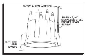
Figure 9 Optional Installation by Bolting Cap Down.
