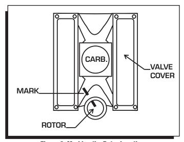
**Figure 8 Marking the Rotor Location.**
