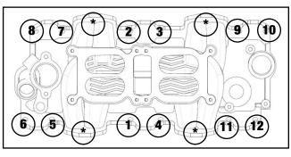
Single & Dual Quad Intake Manifold Torque Sequence
