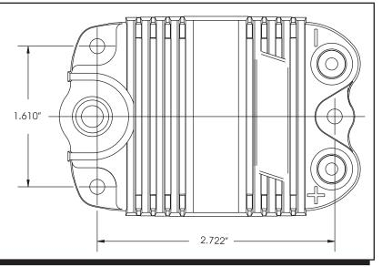
Figure 5 Mounting Template.
