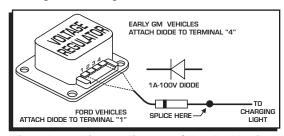
Figure 8 Installing the diode to a GM or Ford Vehicle.
