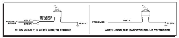
Figure 3 Connecting a Theft Deterrent Switch Through the MSD Ignition.
