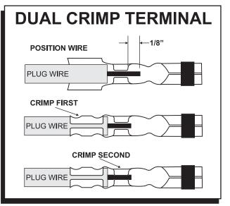
Figure 12 Crimping a Dual Crimp Terminal.
