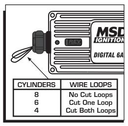
Figure 1 Programming the Number of Cylinders.
