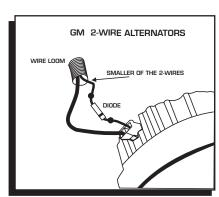
Figure 9 Installing the Diode to a 1973-1983 GM Vehicle.
