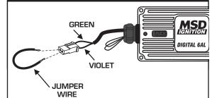
Figure 11 Checking for Spark with the Mag Pickup.
