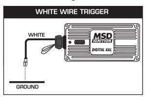
Figure 10 Checking for Spark with the White Wire.
