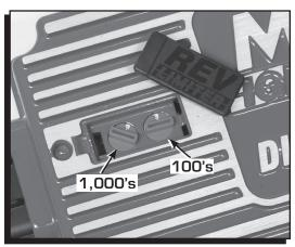
Figure 2 Adjusting the Rev Limits.
