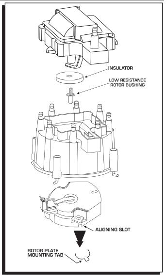
Figure 4 Installing the Modified Dust Cover.
