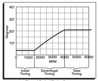
Figure 1 Typical Timing Curve.
