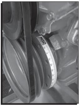
Figure 2 The Timing Tape Installed.
