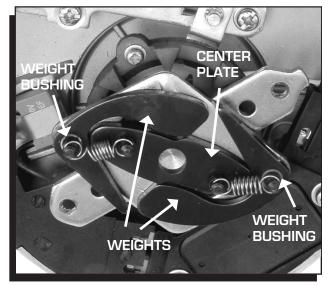
Figure 2 Installing the Advance Kit.
