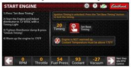
Start the engine and adjust the throttle body screw, as needed, to maintain idle.
