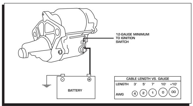
Figure 1 Wiring the Starter.
