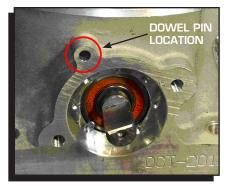
Figure 1 Dowel Pin Location.
