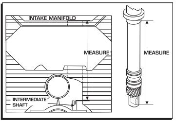
Figure 3 Checking Oil Pump Shaft to the Distributor Shaft Overlay.
