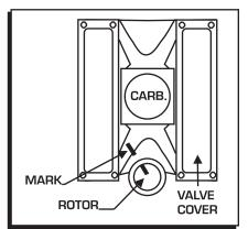
Figure 2 Marking the Rotor Location.
