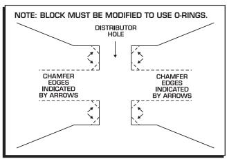
Figure 1 Modified Block to Accept the O-Ring Seals.
