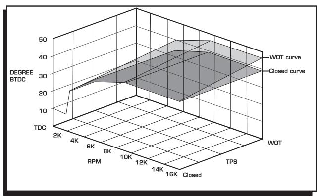
Figure 1 TPS/Timing Curve Example.
