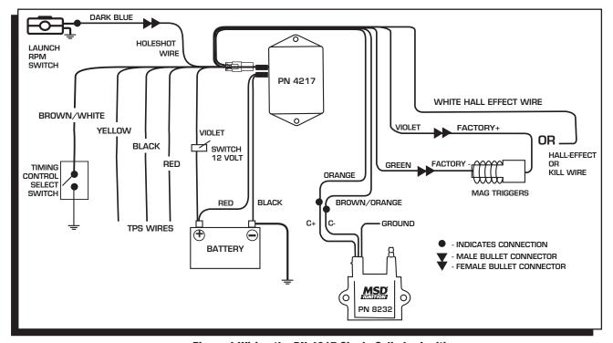
Figure 4 Wiring the PN 4217 Single Cylinder Ignition.
