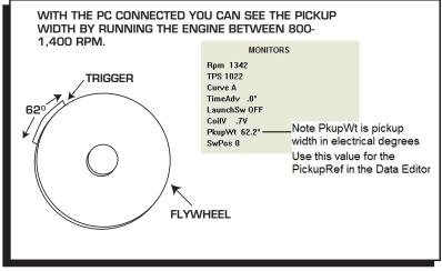
Figure 2 Pickup Width.
