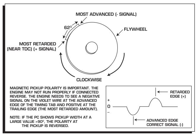
Figure 3 Pickup Polarity.
