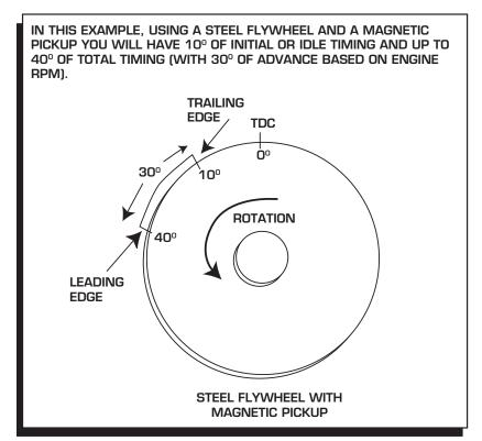
Figure 7 Magnetic Pickup.
