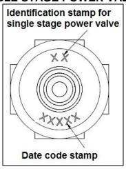
Example: If your current power valve is stamped 12, Holley suggests replacing it with a power valve stamped 65.
