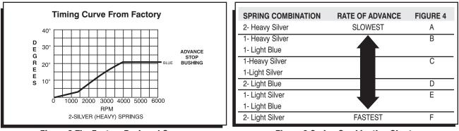
Figure 2 The Factory Equipped Curve.
