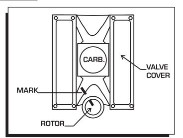
Figure 8 Marking the Rotor Location.
