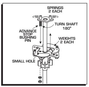
Figure 7 Locking Out the Advance.
