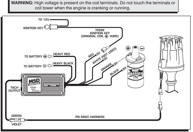
Figure 9 Wiring to an MSD 6 Series Ignition Control.
