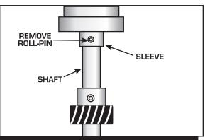
Figure 7 Removing the Retaining Sleeve.
