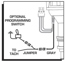
Figure 15 Setting the Rev Limiter.
