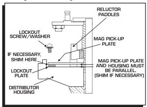
Figure 11 Checking Installation of the Lockout Plate.
