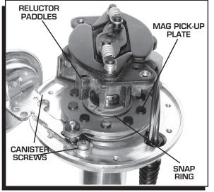
Figure 10 Removing the Vacuum Canister.
