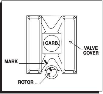
Figure 12 Marking the Rotor Location.
