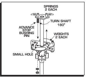
Figure 8 Locking Out the Centrifugal Advance.
