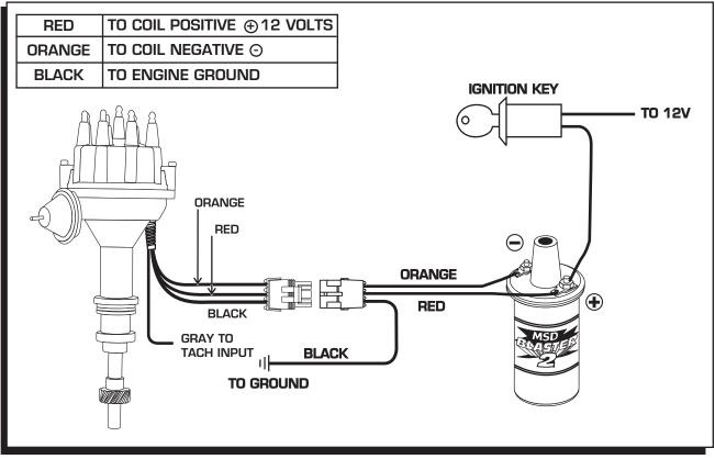
Figure 13 Wiring the Ready-to-Run Ford Distributor.
