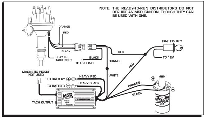
Figure 14 Connecting an MSD Ignition Control.
