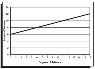
Figure 9 Vacuum Advance and Timing Chart.
