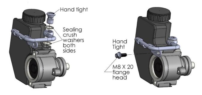
**NOTE:** After assembly torque M8 bolts to 18 ft./lbs. and banjo bolt to 25 ft./lbs.
