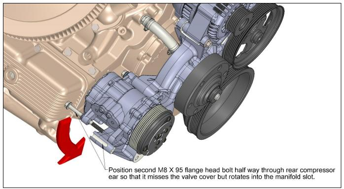
NOTE: After assembly, torque both M8 bolts to 18 ft./lbs.
