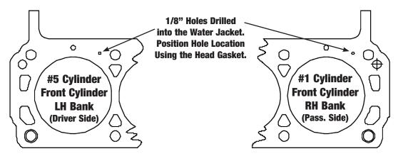
Figure 2 - Steam Hole Locations for Early 289 & 302 Engine Blocks (Pre-1972)
