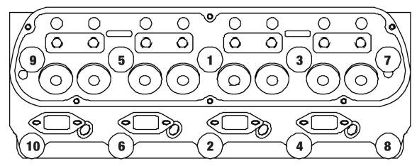
Figure 1 - Head Bolt Tightening Sequence
