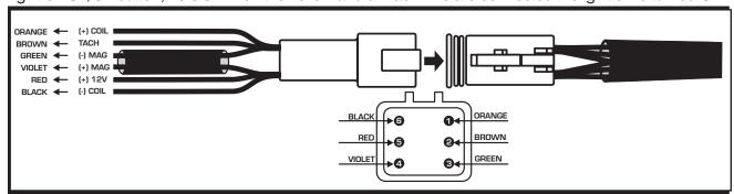
Figure 1 Wire Functions of the 6-pin Connector.
