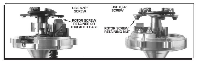
Figure 1 Determining Rotor Screw Length.
