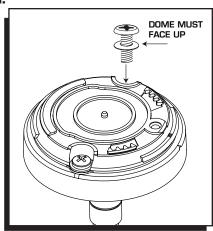
Figure 2 Washer Installation.
