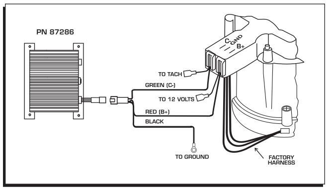
Figure 2 Wiring the PN 87286.
